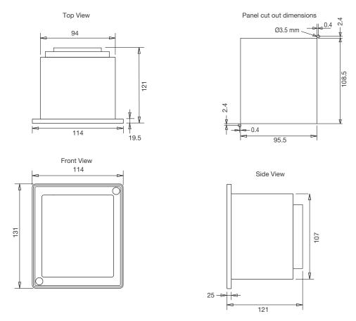
Three Element / Remote Reset (Large Size Enclosure) Relay
