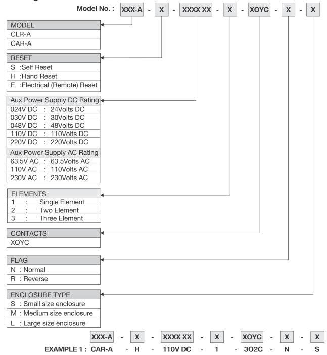
110V DC Relay CAR-A type, Self reset, 110V DC, Three element, Contacts 6 NO / 6 NC and Normal flag in large enclosure.
